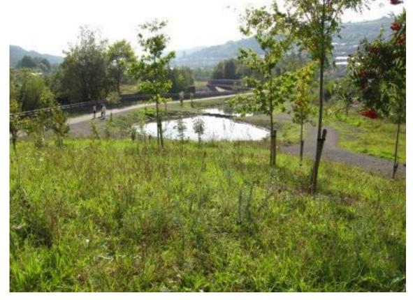
The more informal footpaths have been surfaced with stone dust whilst the main footpaths have been surfaced with macadam. Edging details include engineering brick, PCC kerbs and timber edge boards. Over 275 lm of steel handrailing has been fabricated and installed.
